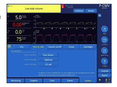
When calibrating the paediatric/adult flow sensor the flow sensor will need to be reversed. The timing of this is indicated in the left upper screen. There should be a frosted piece of tubing available to allow reversal.
